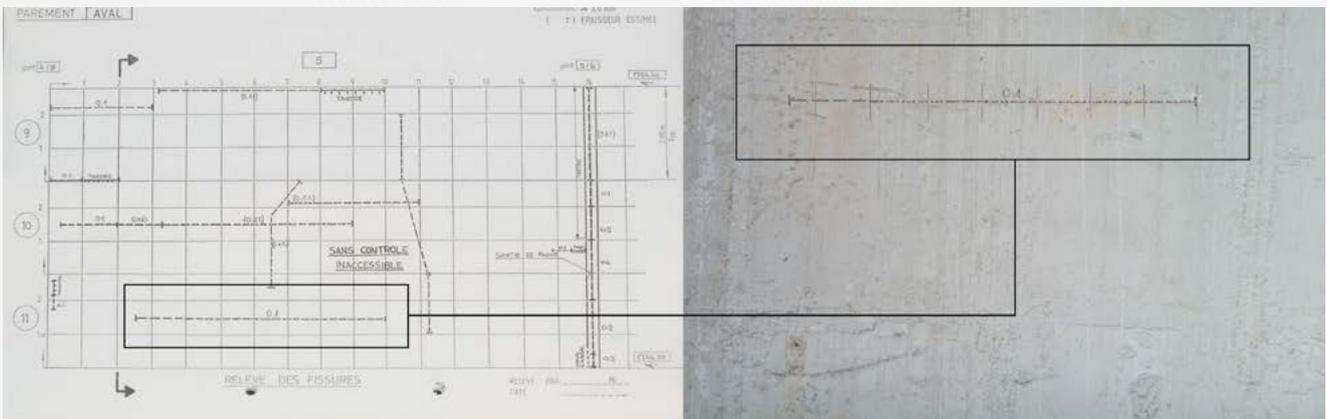
Before and after — a 0.1 mm-wide crack on the dam's face, shown both on one of the drone's photos of this region, and below that on Electricité de la Lienné's historical hand-annotated defect report.
