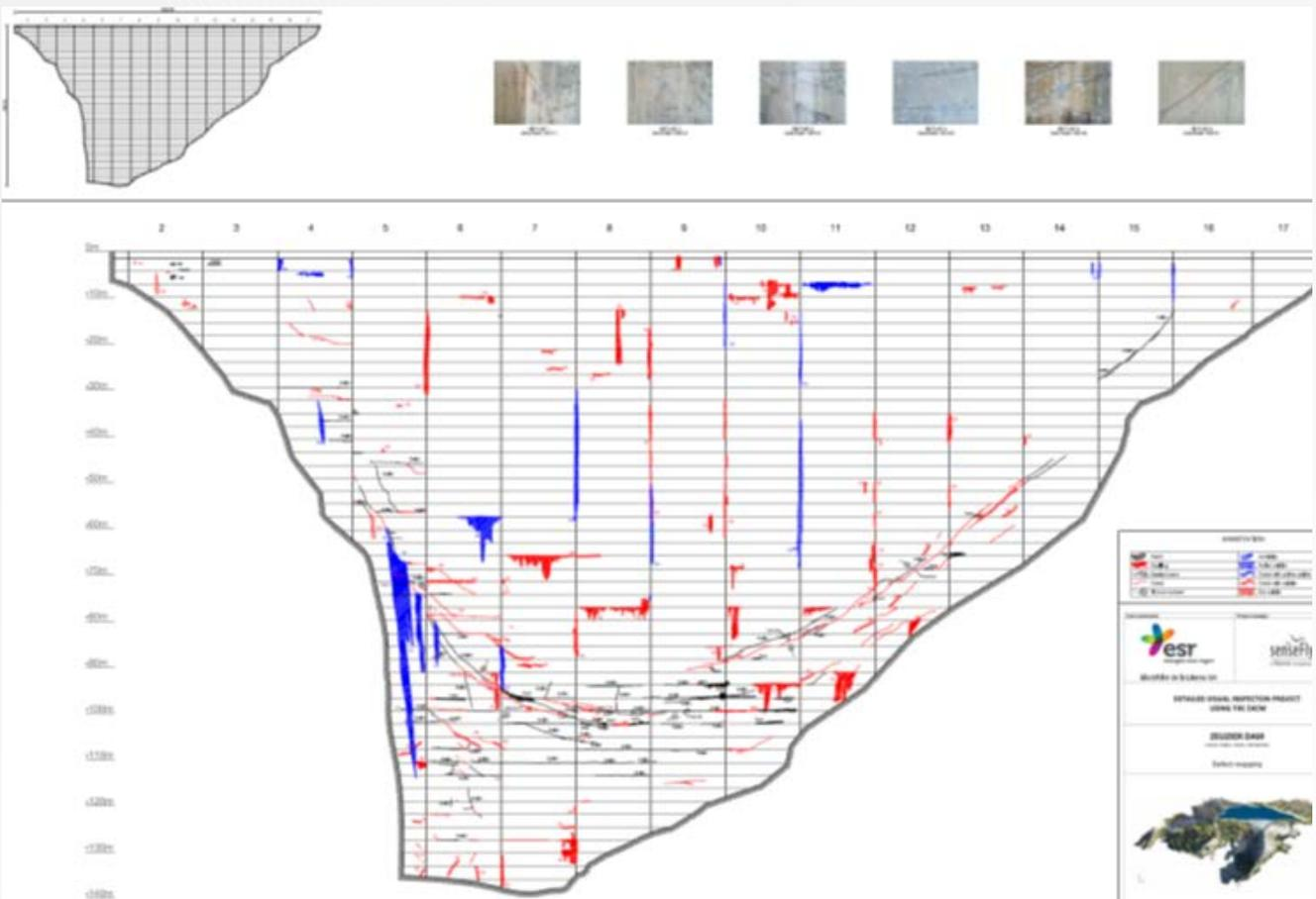
The defect map of the dam's downstream face, produced by senseFly's civil engineer for Electricité de la Lienne.
