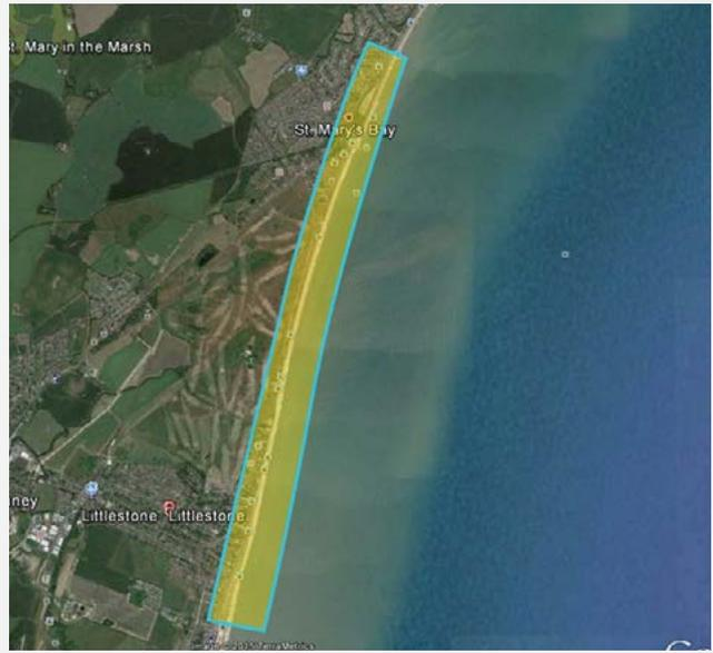
In order to cover the project's 0.5 km<sup>2</sup> at the 2.8 cm/pixel ground resolution required, ATEC-3D's team programmed four 30-minute eBee flights.
