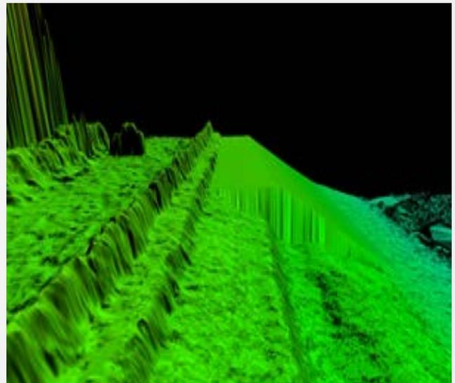
One of ATEC-3D's 3D models, showing one chainage's target profile (background) and its current profile (foreground), the sea wall running up from the bottom-left corner.
