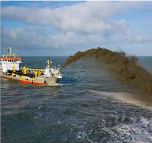
A ship similar to that used by the Environment Agency's replenishment contractor. Its role was to spray shingle onto different 'chainages' (sections of beach) in line with ATEC-3D's volume findings. (Image: Boskalis Westminster.)
