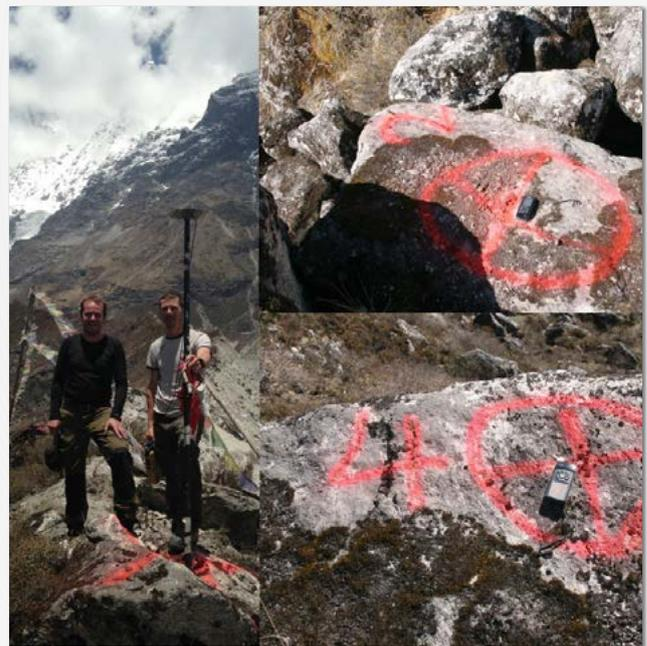
Placing and measuring ground control points using the dGPS. (Images: Steven de Jong)
