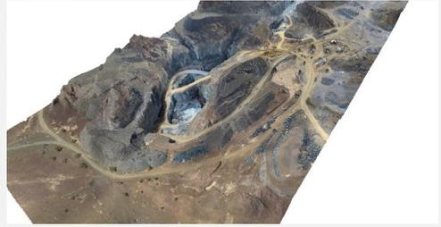
The Al Ram Chromite Mine's final 3D DEM with overlaid orthophoto.
