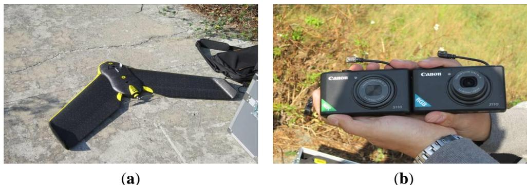
**Figure 3.** UAV imagery system: (a) Fixed-wing UAV; (b) RGB (right) and NIR (left) sensors.
