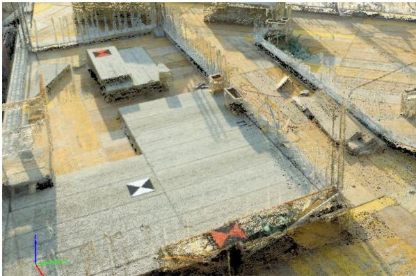
Figure 11 – A close-up of the same densified 3D point cloud with one GCP (black & white) and two check points (red & black) visible.
