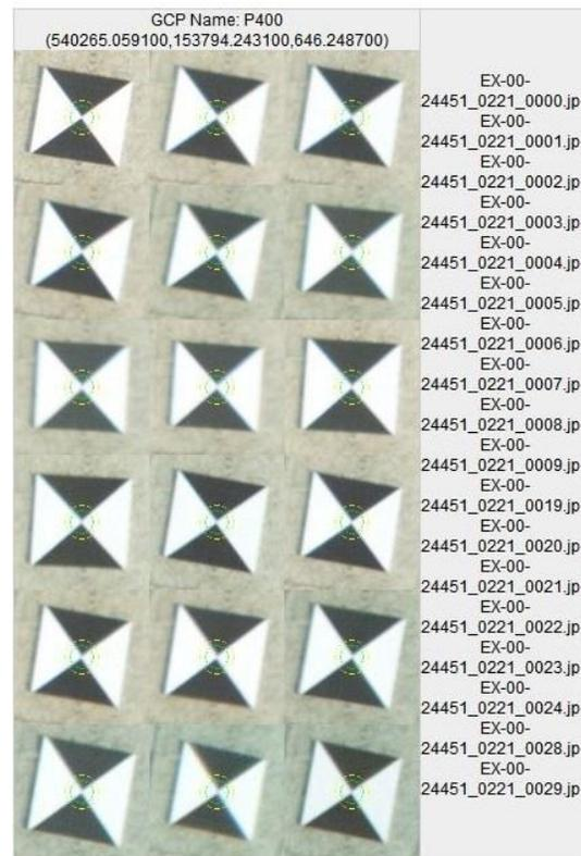
Figure 5 – GCP 400, visible in 18 different images.
