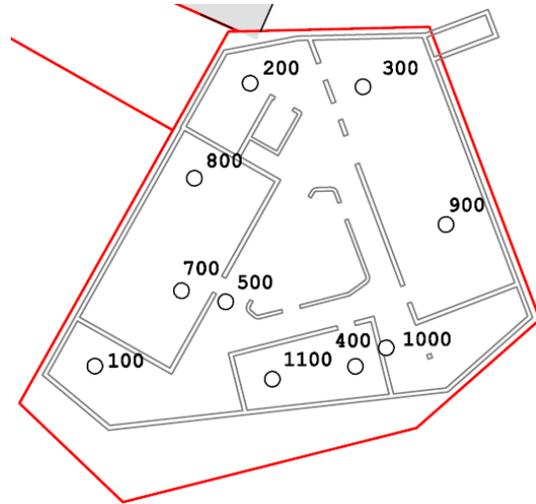
Figure 2 – Map of the ten target positions around the site (in the later processing, numbers 100-500 were marked as GCPs, and 700-1100 were designated as check points).
