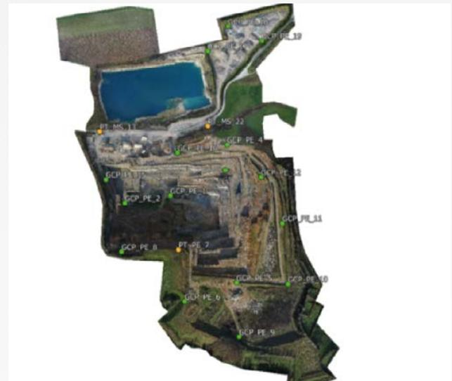
An orthophoto of a Groupe CB quarry, showing the distribution of Redbird-installed GCPs.
