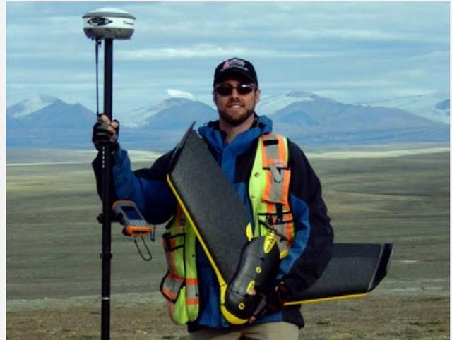
Yannick Lanthier of BluMetric Environmental Inc. with the project's two surveying instruments: a senseFly eBee drone and an RTK GPS.
