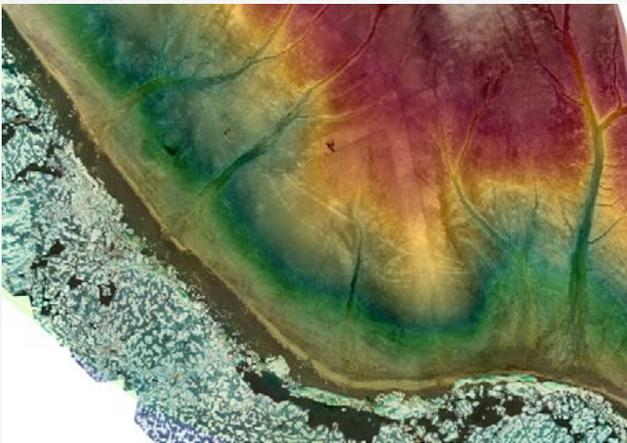
A digital elevation model of a contaminated exploration site on a Nunavut island, layered on top of the team's orthophoto of the site. "We can see the site features old runways that were used by the exploration companies back in the 1970's, major drainage paths/ rivers, the contaminated site to the West and the impressive ice barrier along the coast," Lanthier explains.
