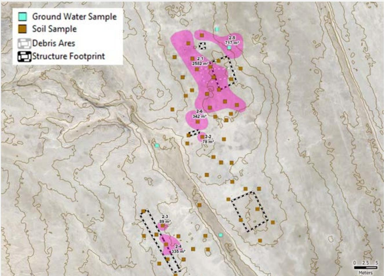
A BluMetric map of one small part of a site showing contaminated zones in pink, with sampling points, structures and a debris zone also noted.
