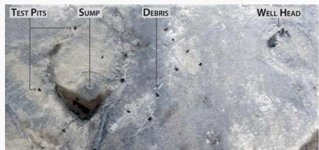
A drone-produced orthomosaic of an old exploration site, featuring a test pit, well head, sump and debris.
